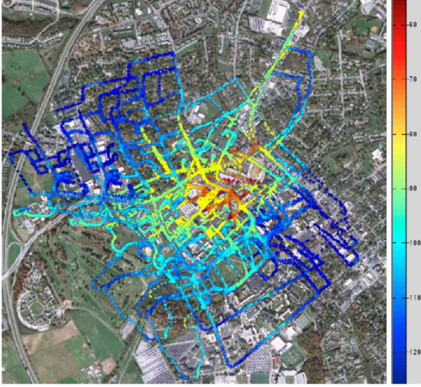
Figure 2: Heat Map of RSS Measurements (in dBm).
